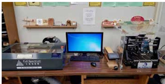
**Figure 2.** Laser and CNC station. Photo Credit: University of Maryland Eastern Shore, Department of Technology.
