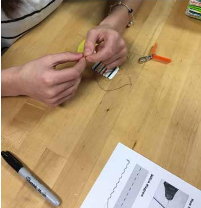
**Figure 2.** Student threading a sewing needle with conductive thread to make a wearable electronic device.
