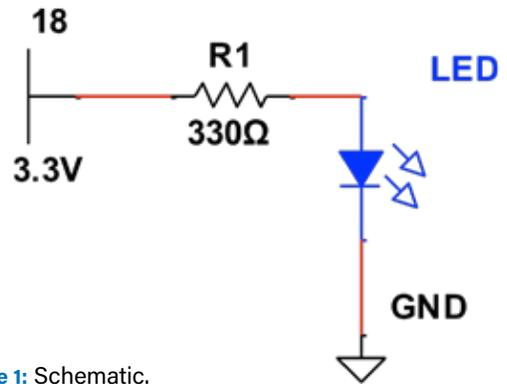
Figure 1: Schematic.
