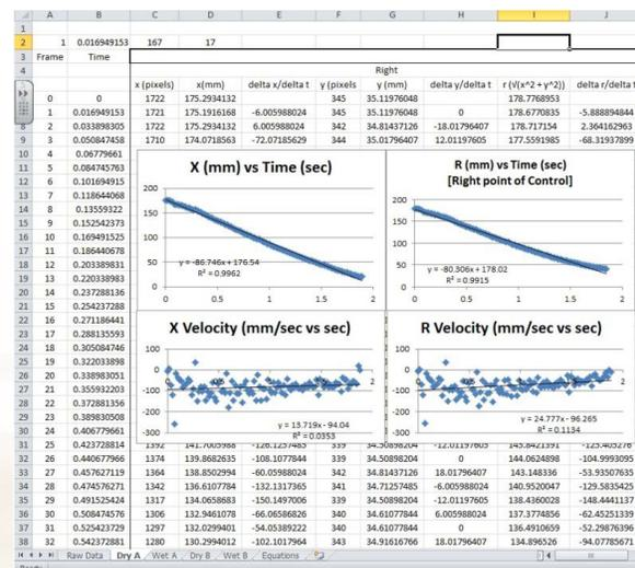
Example of data sheet and plotted data for Dry A trial, right point of control.
